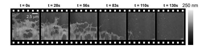
Scanning ion conductance microscopy (SICM) reveals the surface topography of samples without damaging them. This technique measures the current of ions flowing between the probe — an electrolyte-filled pipette — and an electrode in the bath surrounding the sample. When the pipette tip nears the sample surface, ion conductance around the tip changes. Researchers can look at this change in the ion conductance to image a sample's surface without direct physical contact.
