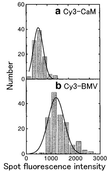
**FIG. 1.** Distributions of spot intensities (arbitrary units) for (a) Cy3-CaM and (b) Cy3-BMV. The spot intensities were obtained by integrating the intensity over a square (13  $\times$  13 pixels) enclosing the spot and subtracting a background integrated over the same square after complete photobleaching of Cy3.
