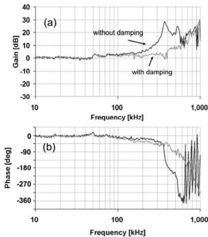
Fig. 8. Frequency spectra of mechanical response of the z-scanner. (a) Gain spectra, (b) phase spectra. Black-line curves represent the responses without feedforward active damping, and gray-line curves represents the responses with feedforward active damping.
