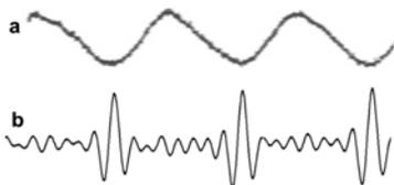
Fig. 11. Force signal (b) calculated from the oscillation signal (a) of a cantilever interacting with a mica surface in water.
