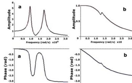
Fig.6. Effect of feedback control for active damping on the resonant system that consists of two elemental resonators connected in parallel. This effect was theoretically calculated. (a) Bode plots of the resonant system before damping. (b) Bode plots of the resonant system after damping.
