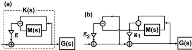
Fig. 7. Circuit diagram for APITF.  $G(s)$  represents a given transfer function for a real resonant system.  $M(s)$  represents a transfer function of a mock resonator for  $G(s)$ . (a) Single-loop circuit type.  $K(s)$  approximately gives  $1/M(s)$ . (b) Nested circuits for improving the approximation.
