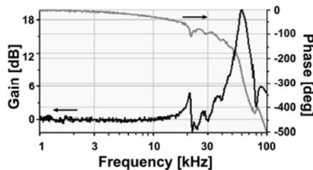
Fig. 2. Frequency spectra of mechanical response of the x-scanner.
