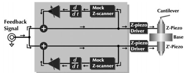
Fig.4. Active Q-controller for the z-scanner. The mock z-scanners are RLC circuits characterized with the transfer functions similar to those of z- and z'-scanners.
