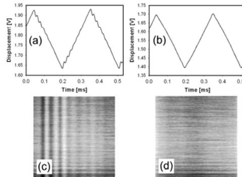
Fig. 3: Effect of feedforward active-damping control on the x-scanner vibrations. (a) X-scanner displacement driven by triangle waves without damping. (b) X-scanner displacement driven by triangle waves compensated by the feedforward control. (c) Mica surface images acquired at 33 frames/s without and (d) with damping.
