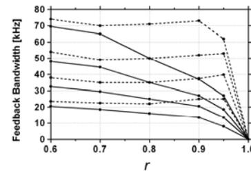
Fig. 9. Feedback bandwidth as a function of the set point  $r$ . Solid-line curves: feedback bandwidths measured with a conventional PID controller; dotted-line curves: feedback bandwidths measured with the dynamic PID controller. These curves are aligned from top to bottom according to the ratio  $2A_0/h_0 = 5, 2, 1$ , and  $0.5$ .
