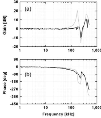
Fig. 5. Frequency spectra of mechanical response of the z-scanner. (a) Gain spectra, (b) phase spectra. The gray-line curves represent the response without feedback Q-control, and the black-line curves represent the response with feedback Q-control.
