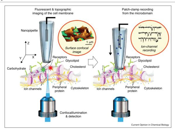
Scanning ion conductance microscopy can be combined with confocal fluorescence imaging to obtain simultaneous topographic and fluorescence images of the cell surface. The same nanopipette can be used to image function by detecting ion channels in the cell membrane.
