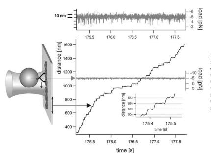
from  $\sim 11$  nm for applied loads of 0.7 pN to  $\sim 4$  nm at 5 pN. The standard deviation of the free bead position signal at a spring constant of 0.02 pN/nm was  $\sim 14$  nm.
