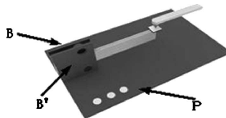
FIG. 1. Schematic diagram of the cantilevered bimorph-based scanner for high speed scanning.
