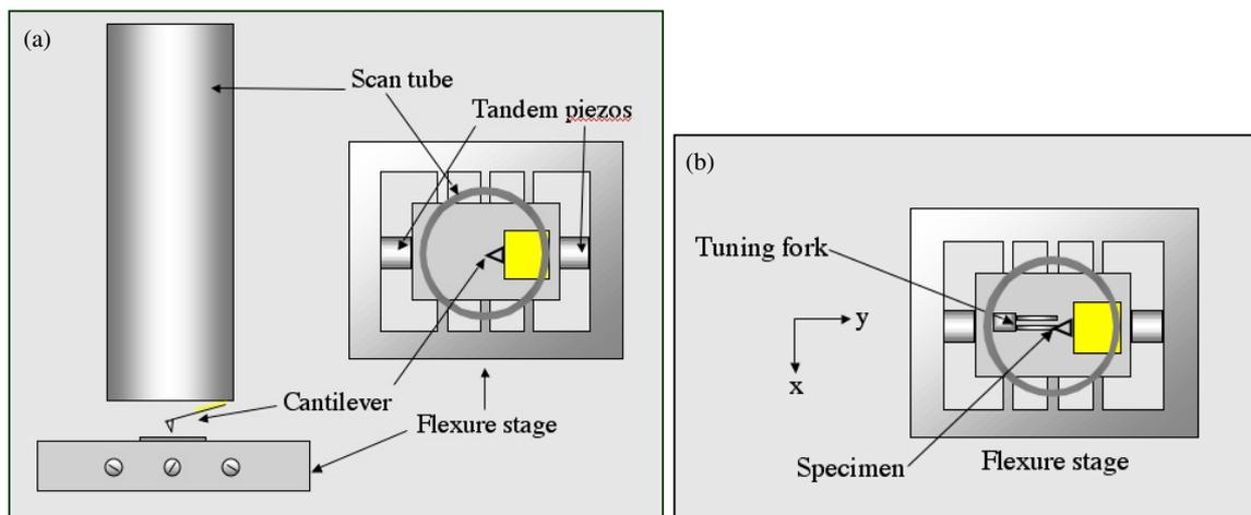
**Figure 1.** (a) Position of the high-speed flexure scanning stage in relation to a micro cantilever mounted on the scan tube, and, (b), for kilohertz frame rates a high speed tuning fork scanner was mounted on the flexure stage that provided the slow scan direction. (This figure is in colour only in the electronic version)
