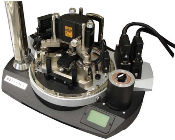
Fig. 1. The NT-MDT Ntegra scanning probe microscope arranged in scan-by-probe configuration. The scan head is mounted above a stationary sample platform.
