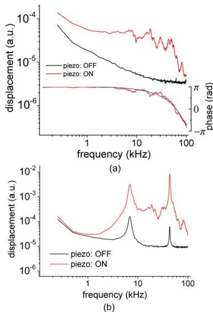
FIG. 3. (Color online) Frequency response of (a) a cantilever chip (b) a cantilever (Veeco MLCT-C) measured using an AFM system (Veeco Dimension 3100). The seesaw holder was put onto the pins of the AFM head. The optical lever sensor of the AFM system was used to gather data when the seesaw holder's piezo was turned off and on. The piezo actuator was driven with a white noise.
