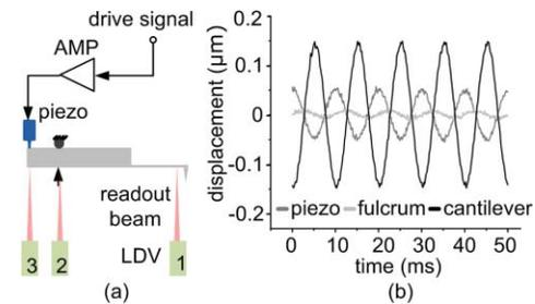
FIG. 2. (Color online) (a) Schematic view of the optical setup using a laser Doppler vibrometer (LDV) to characterize the seesaw actuation holder. *Point 1* represents the piezo readout location, *Point 2* represents the fulcrum readout location, and *Point 3* represents the cantilever readout location. (b) Displacement data measured by LDV at three different positions along the cantilever chip at a V<sub>p-p</sub> signal of 5 V.
