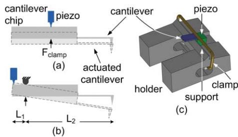
FIG. 1. (Color online) (a) Schematic view of a conventional method of actuating an AFM cantilever. Piezo actuator simply translates the cantilever in vertical direction. (b) Schematic view of proposed method of actuation. Piezo actuator translates the end of the cantilever chip. The chip is free to rotate along the out-of-plane axis passing through the support point. (c) 3D model of a cantilever holder employing seesaw actuation method.
