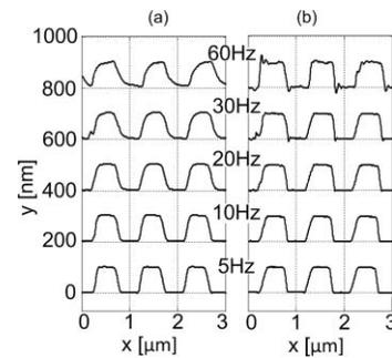
FIG. 4. Contact-mode line scans of a calibration sample obtained at different speeds. The sample was imaged using (a) the z-piezo of the commercial AFM system and (b) the seesaw holder with the same feedback settings. The calibration sample is a 100-nm-thick diffraction grating with a period of  $1\ \mu\text{m}$ .
