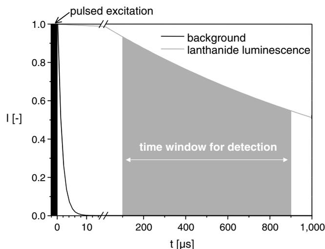
**Fig. 3** Principle of time-resolved luminescence measurements
