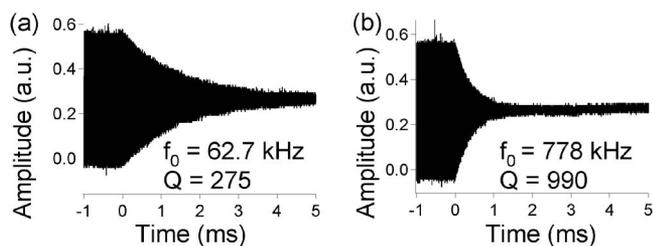
FIG. 2. Amplitude decay of (a) flexurally oscillating and (b) torsionally oscillating T-shaped cantilever after the drive signal is switched off at  $t=0$ . The times taken for the amplitudes to decay to  $1/e$  of their initial values are approximately 1.4 and 0.4 ms, respectively. These values match the decay time calculated from the resonant frequency and  $Q$  (shown) of the respective mode used.
