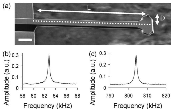
FIG. 1. (a) Scanning electron micrograph of T-shaped cantilevers used in this work (Mikromasch TL01), showing the cantilever length ( $l$ ) and tip offset ( $d$ ). The dotted line marks the torsion axis. Scale bar  $10\ \mu\text{m}$ . (b) The first flexural and (c) torsional resonances of a T-shaped cantilever. The resonant frequencies are 62.8 and 804 kHz and quality factors are 150 and 672, respectively.
