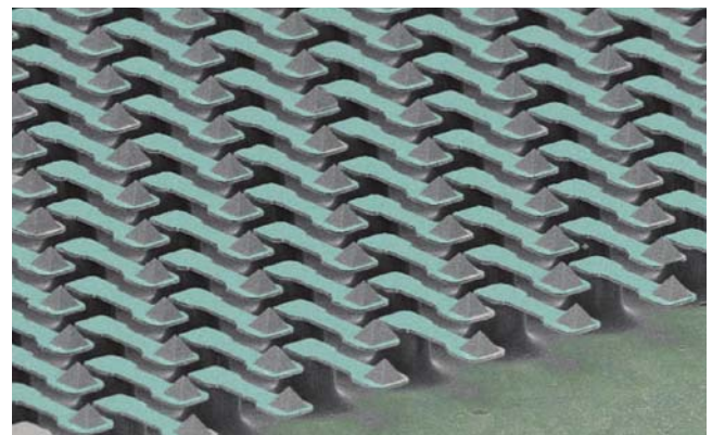
Fig. 3 Scanning probes with undesirable intrinsic bending.
