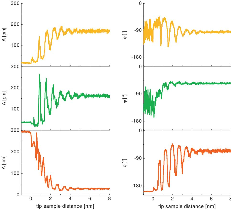
FIG. 1. (Color) Amplitude and phase of the AFM cantilever vs separation between the solid HOPG surface and the cantilever tip for different drive frequencies [top/yellow: 41 kHz ( $\omega/\omega_0=0.95$ ), middle/green: 32 kHz ( $\omega/\omega_0=0.75$ ), and bottom/red: 6 kHz ( $\omega/\omega_0=0.15$ ) relative to resonance (43 kHz). The periodicity of the oscillations reflects the size of the molecules (OMCTS).
