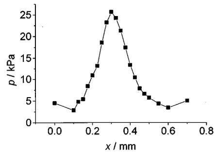
FIG. 3. Measured pressure amplitude of the sound wave transmitted through a slit 50  $\mu\text{m}$  wide.
