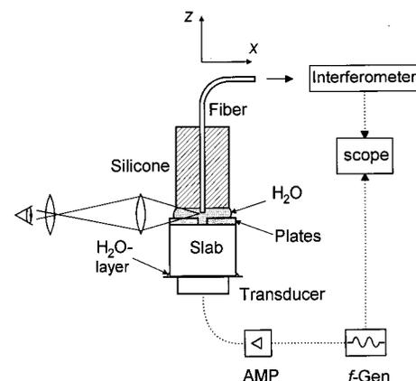
FIG. 1. Experimental setup of the transmission microscope configuration; f-Gen: function generator; AMP: amplifier.
