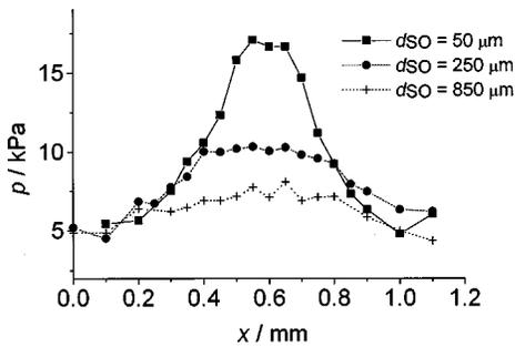
FIG. 2. Measured pressure amplitude of the sound wave transmitted through a slit 0.2 mm wide vs distance in the scanning direction dependent on the sensor-object distance  $d_{SO}$ .
