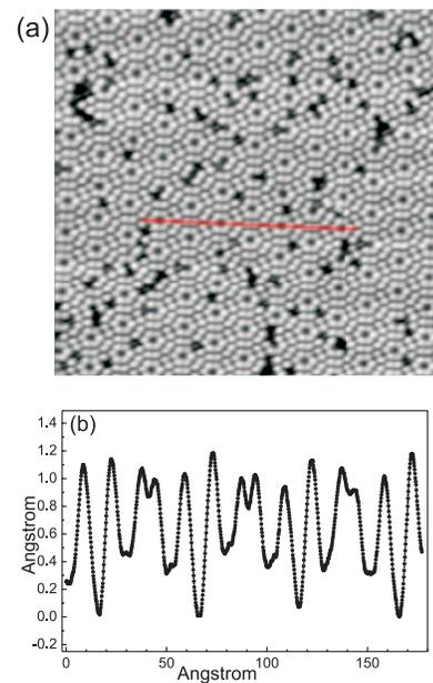
FIG. 5. (Color online) (a) Atomsically resolved unfiltered STM image of the  $(7\times 7)$  structure on a Si(111) sample (lateral scan size  $30\text{ nm} \times 30\text{ nm}$ ). (b) Line scan (not averaged) through the red line in (a).
